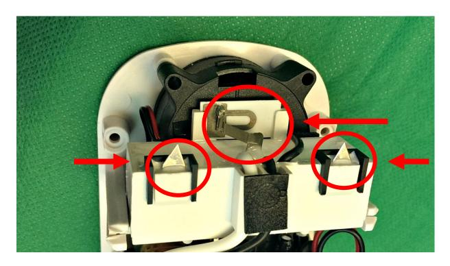
**Step 4: Wipe parts clean.** Dip new cotton swab in rubbing alcohol. Carefully clean metal tips. Thoroughly clean plate. (See items above circled in red).
