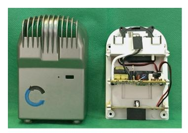
**Step 3: Clean casing.** Dip cotton swab in rubbing alcohol and wipe between spaces of outside cover. Also clear any debris from the inside of the cover.
